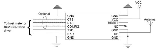
See page 19 for additional schematic information regarding recommended Reset and Power supply filtering, and how to include a firmware upgrade connector.
