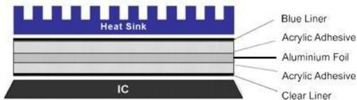
All ABL's BGA heatsinks are supplied with thermal tape.
