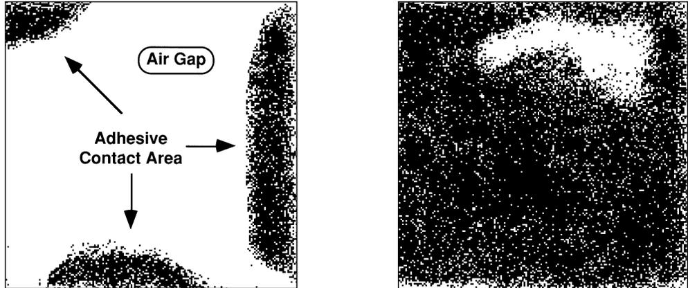
Choice of adhesive thickness well exceeding the runout of flatness on the part (especially rigid substrates), coupled with optimal assembly methods can help reduce air gaps (as discussed in Section I) and increase the high temperature reliability.
