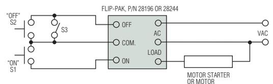
With two normally open, momentary contact push buttons (S1 and S2), the **FLIP-PAK** provides solid-state control of the motor starter or the motor itself... if load requirements are within FLIP-PAK ratings. S3 provides a safety shut-down. With S3 closed, the “ON” push button (S1) is rendered ineffective by the “OFF” override feature of the FLIP-PAK.
