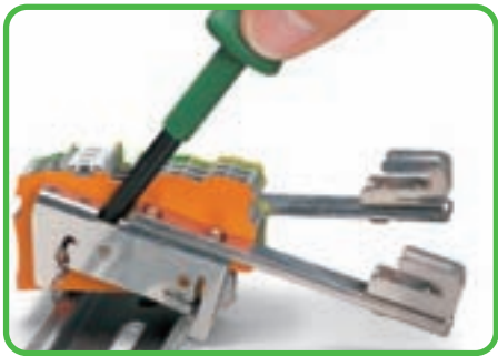
Remove the busbar carrier using a screwdriver (blade width 5.5 mm / 0.217 in)
