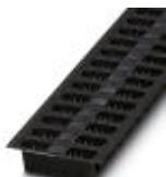
Header, Nominal current: 8 A, Rated voltage (III/2): 250 V, Number of positions: 2, Pitch: 3.5 mm, Color: black, Contact surface: Tin, Mounting: THR soldering, The maximum current depends on the plug used. The lower of the two current values apply for plug and pin strip. The pin strip is made of highly temperature resistant plastic and is thus suitable for the reflow process.
