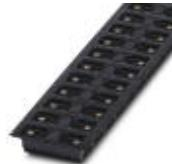
Header, Nominal current: 8 A, Rated voltage (III/2): 160 V, Number of positions: 3, Pitch: 3.5 mm, Color: black, Contact surface: Tin, Mounting: THR soldering, User information and design recommendations for through hole reflow technology can be found under "Downloads"
