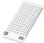
Marker card, Card, white, labeled, Horizontal: Consecutive numbers 1 - 10, 11 - 20, etc. up to 91 - 99, Mounting type: Adhesive, for terminal block width: 3.5 mm, Lettering field: 3.5 x 2.8 mm
