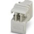
Header, Nominal current: 8 A, Rated voltage (III/2): 160 V, Number of positions: 3, Pitch: 3.5 mm, Color: light gray, Mounting: Soldering, Article with lateral pin exit
