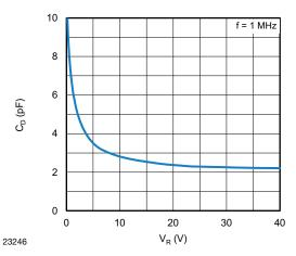
Fig. 4 - Typical Capacitance vs. Reverse Voltage
