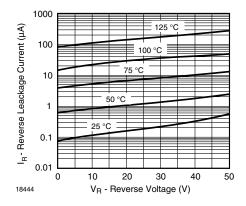
Fig. 3 - Typical Reverse Characteristics
