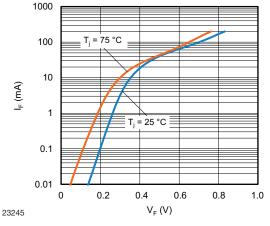
Fig. 2 - Typical Forward Characteristics
