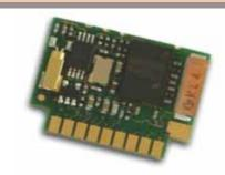
This miniature module enables full duplex Bluetooth® data or audio transmissions over 20m.
