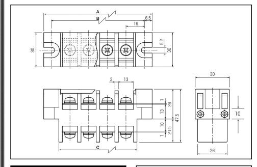
BlockMaster Electronics' new OTB-358 Series are medium-power, thru-panel terminal blocks available in 2-15 positions.
