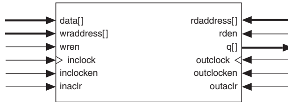
Figure 2–13. Simple Dual-Port & Single-Port Memory Configurations
