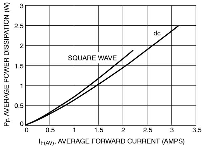
Figure 9. Power Dissipation
