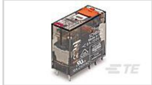
Power Relay Type: **Industrial Panel Plug-In**Coil Magnetic System: **Monostable, DC**Coil Power Rating Class: **400 – 500 mW**Coil Power Rating DC: **419 mW**Coil Resistance: **1440 Ω**
