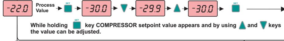
If both **▲** keys are pressed and held for 3 seconds, programming mode is entered.
