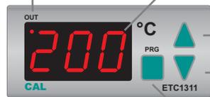
Displayed process value in the run mode, parameter name or value in programming mode.
