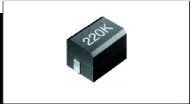
Specially developed for automatic mounting applications, this exciting range of chip inductors are ferrite based and sealed in a thermoset plastic body. They employ solder coated copper terminations with barrier layer. Customers can therefore expect consistent quality, performance and reliability. Its smooth top surface makes it particularly well suited to pick and place equipments.
